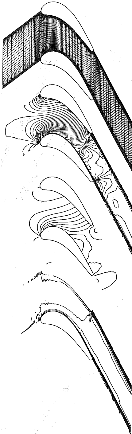
Fig. 10(a) Structured H-mesh for conventional flow solver: The mesh consists of 4950 node points; (b) Mach contours of steady turbulent solution on the structured mesh: The contour interval is 0.025; (c) static pressure contours of steady turbulent solution on the structured mesh: The contour interval is 0.05; (d) entropy contours of steady turbulent solution on the structured mesh: The contour interval is 0.02
